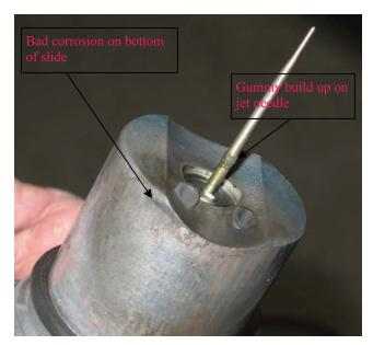
The Bing carb controls fuel mixture by moving a tapered needle (jet needle) into and out of a fixed orifice (needle jet). Engine vacuum is fed to the top side of a diaphragm in the carb dome. When the throttle butterfly (which controls airflow in to the engine) is opened more vacuum reaches the top of the diaphragm pulling it upward.
