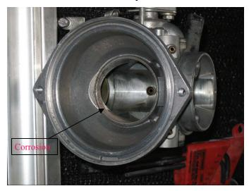
Corrosion was also observed on the carb slide itself (sometimes called piston) as well as some buildup of a varnish like substance.
